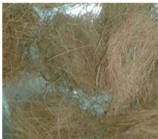
(1a). Natural coconut fiber used to make ECC concrete.
