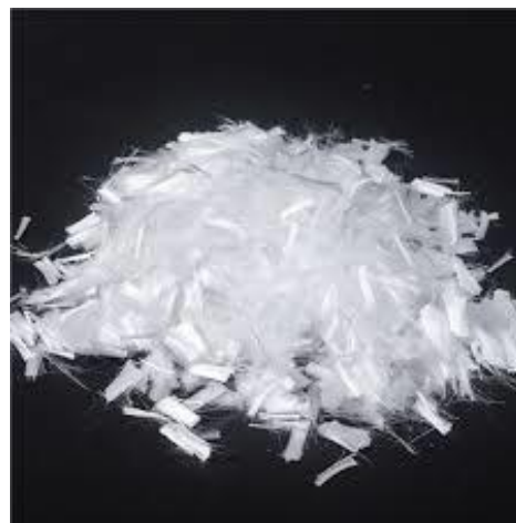
(1b). PVA fiber has the size 6 and 12 mm used to fabricate ECC concrete.
